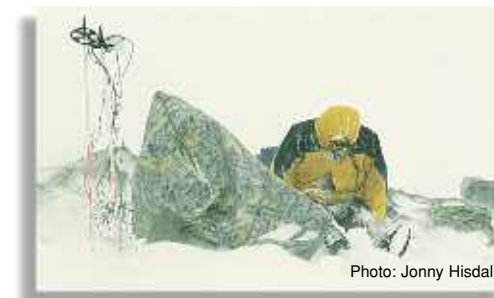
From the field-tests on Snohetta. Notice all the wires to the temperature gauges on the test-person
